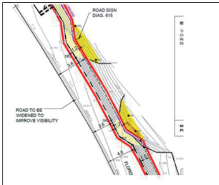
PROPOSED FOOT PATH (red lines) AND SINGLE CARRIAGEWAY ROAD LAYOUT WITH PRIORITY SYSTEM ON FLORDON RD
